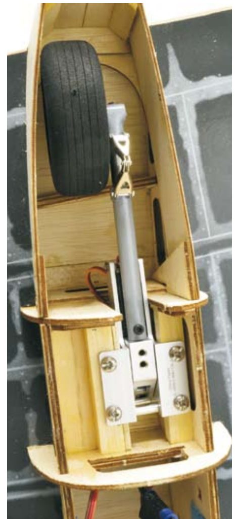
The main retracts, struts and wheels fitted nicely within the nacelle formers with very little work
