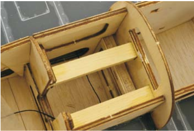
The main retracts, struts and wheels fitted nicely within the nacelle formers with very little work
