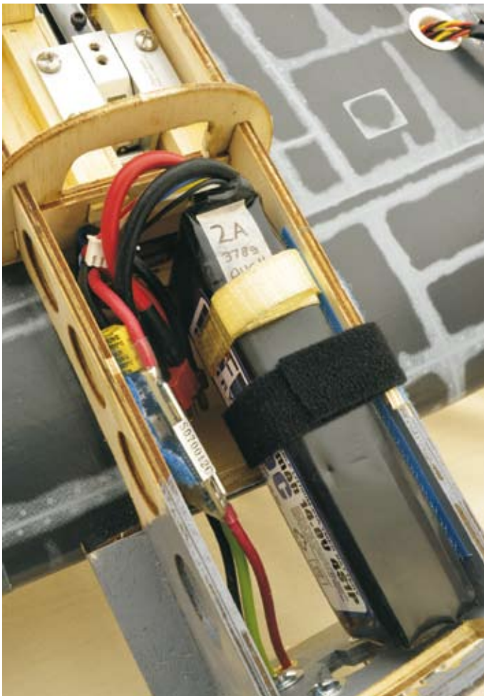
With plenty of room available, the standard sized radio gear was easily installed in the fuselage under the wing. The Castle BEC sits on the redundant flight battery tray
