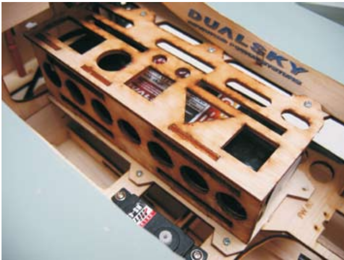
This is the pre-assembled battery box that can be simply screwed into place.
