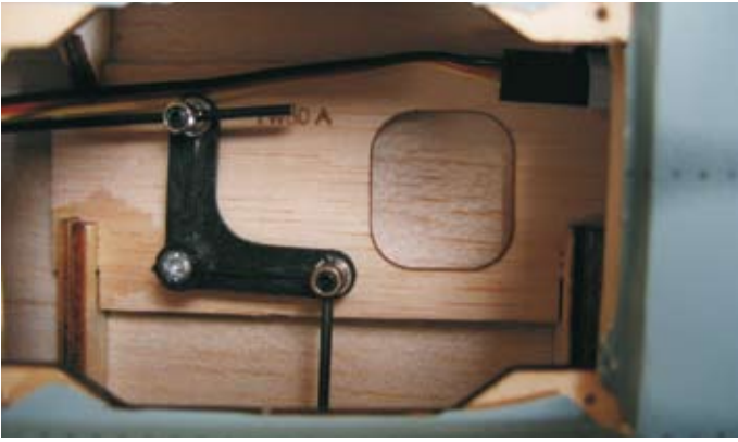
The mechanical flap set up.
