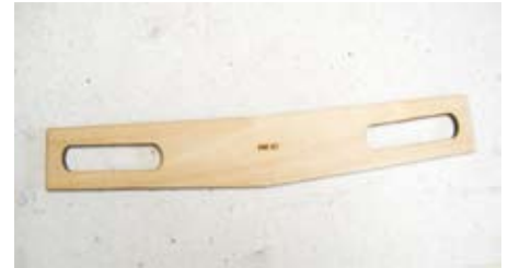
A very substantial ply joiner forms the basis for the robust wings.
