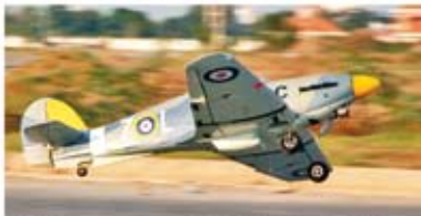
VQ Hawker Hurricane .60 WS: 1.6 m Wt: 3.6 kg Engine: .60 2-st - .91 4-st Radio: 7 CH 7 servos
